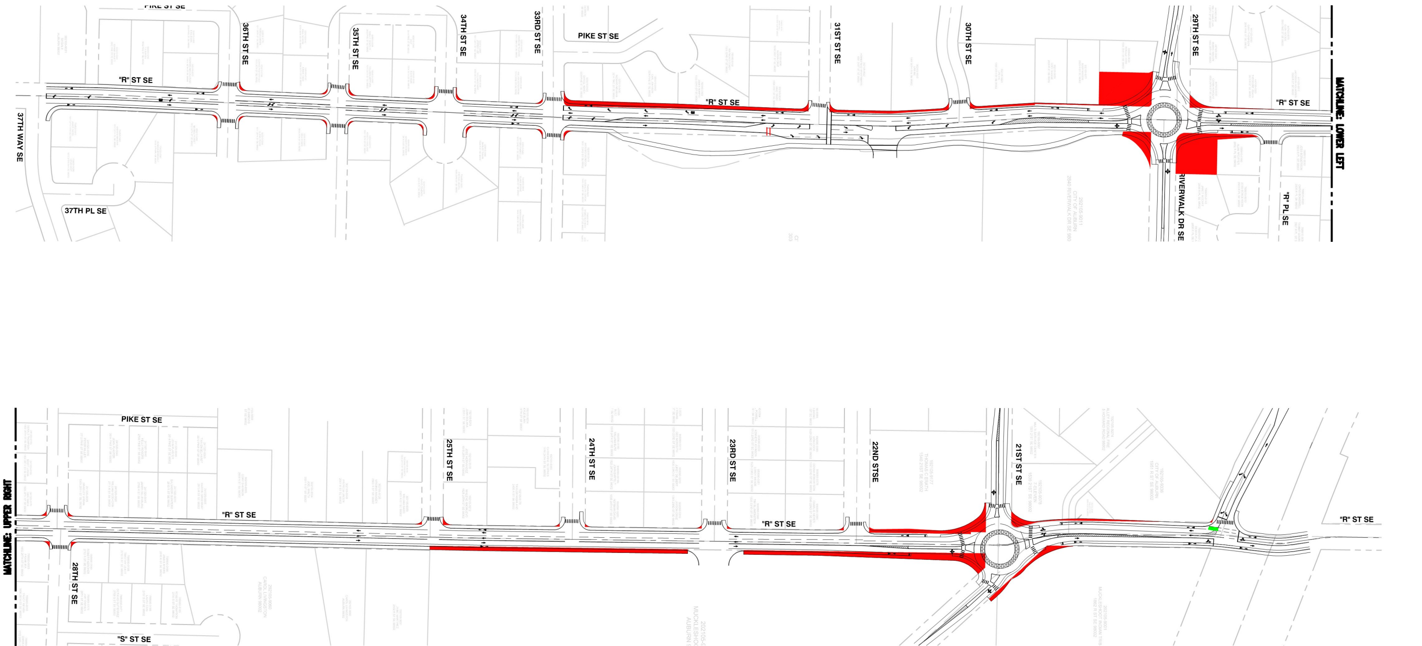
Figure 4B - Alternative 3 with Roundabouts
