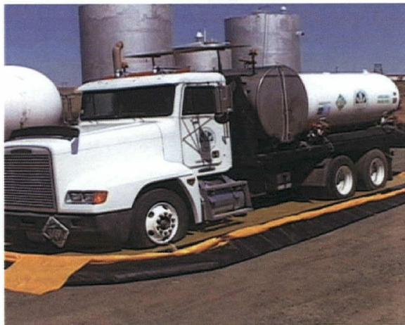
One Type of Pre-fabricated Containment System
