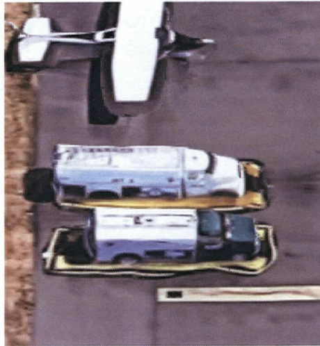
Pre-fabricated Containment @ Arlington Airport
