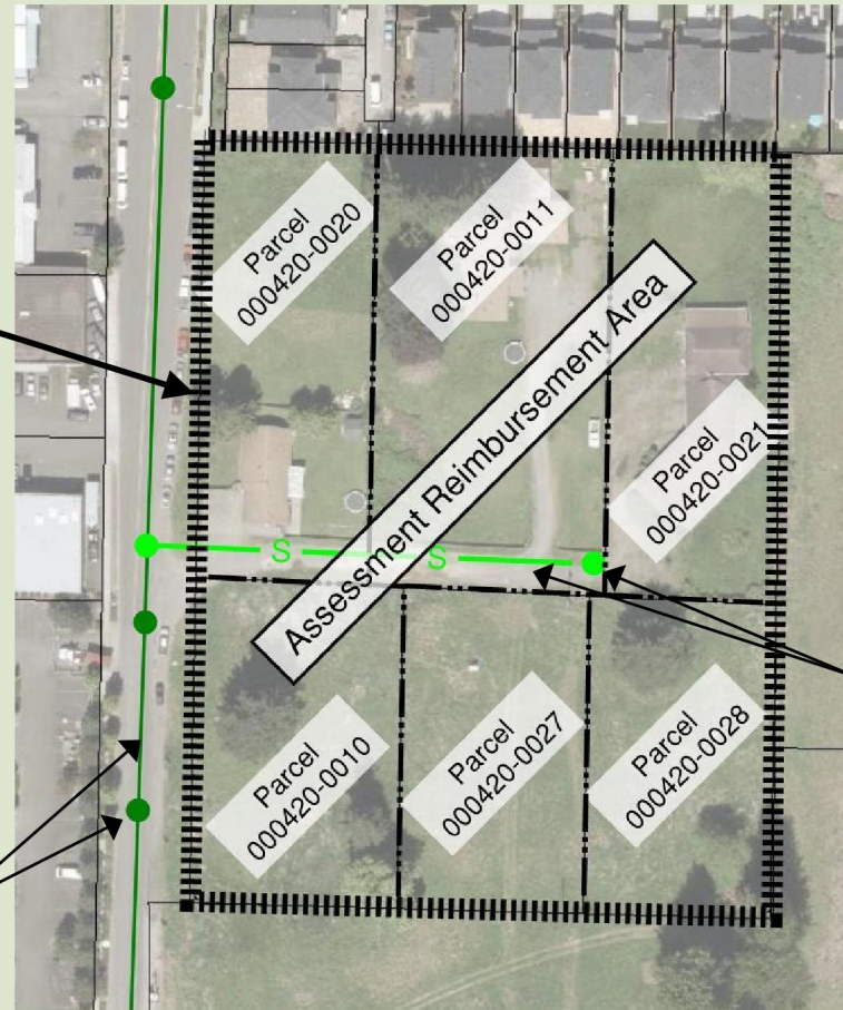
New Sewer Main and Manholes
