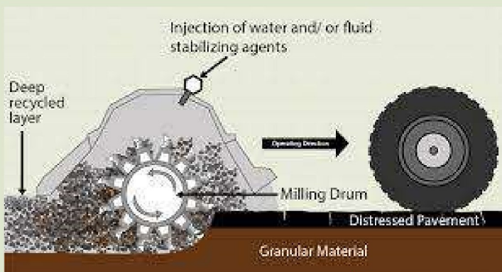
Pulverizing Existing Roadway
